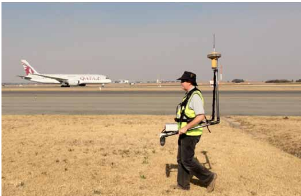
Figure 11 UNISCAN™ deployed on an underground pipeline whose route has already been marked out by a pipe locator.
