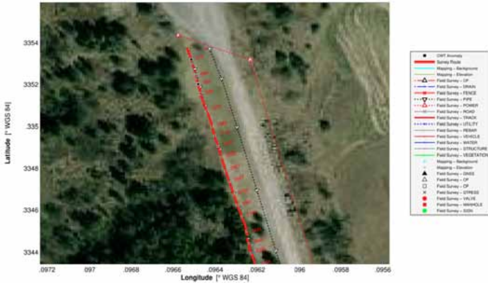
Figure 22 Survey Map showing a portion of the pipeline route inspected by SCT™. The red line shows the survey route, the black dots represent SCZs, the red text by each SCZ is its unique ID which can be cross referenced in both the anomaly table and strip charts. GNSS co-ordinates have been removed to protect client confidentiality.
