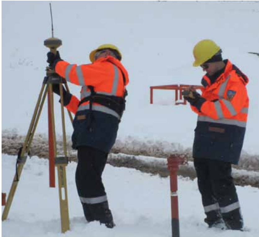
Figure 12 Technicians set up the Base Station to receive signals from GPS and GLONASS satellites and which broadcasts its position to the GNSS receiver attached to the rear of the UNISCAN™ frame.
