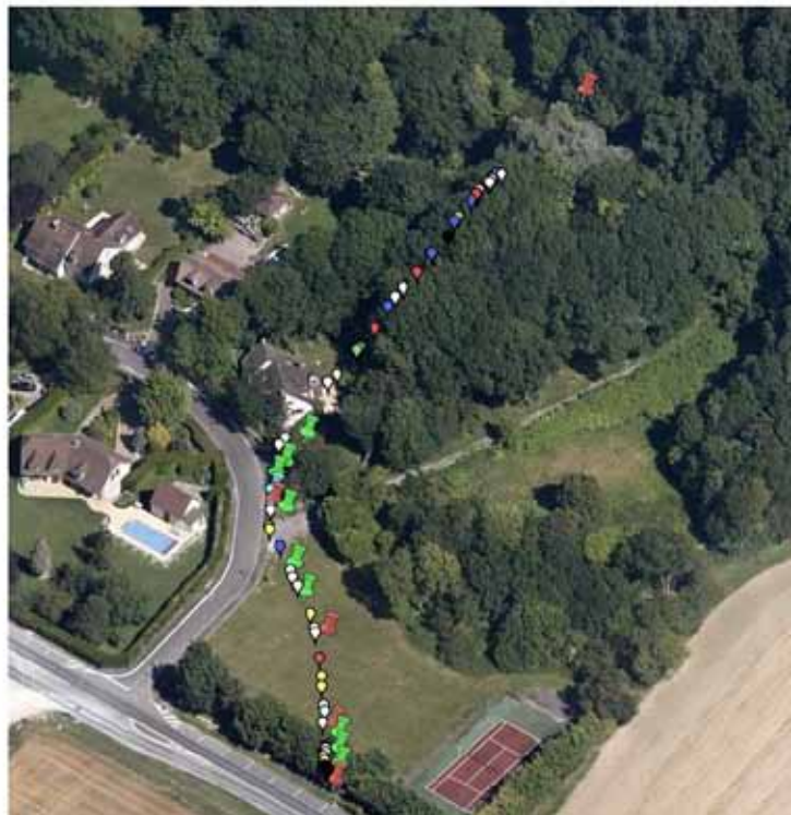
Figure 18 A GIS overlay of SCT and DCVG/CIPS results. SCT data is easily integrated into the datasets of both DCVG/CIPS and ILI results to allow intuitive cross-comparison of data.
