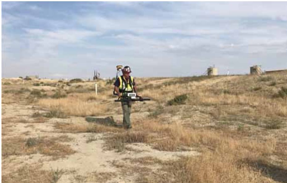
Figure 7 UNISCAN™ deployed on distribution lines at a gas facility in the United States.
