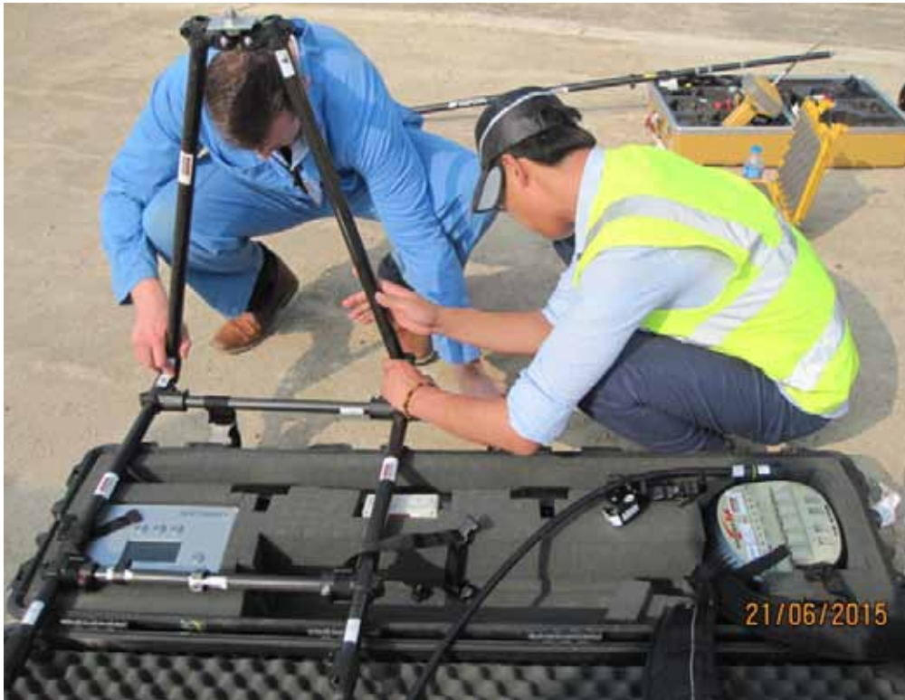
Figure 10 Technicians assembling UNISCAN™. The device is portable and rapidly assembled onsite. Construction takes between 10-15 minutes.
