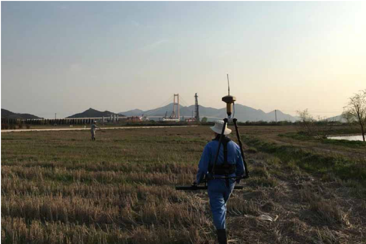
Figure 2 UNISCAN™ scanner deployed in China on transmission line illustrating uninterrupted data collection at normal walking speed.
